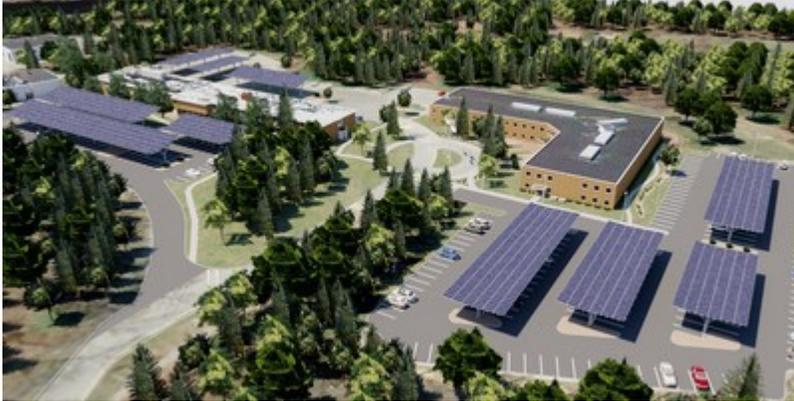
Start of construction is targeted for summer 2019. The integrated solar parking canopy project will feature high-efficiency SunPower® solar panels installed across multiple solar parking canopies, and is expected to produce enough electricity to offset approximately 20 percent of the facility's energy needs thereby reducing Cabot's grid energy costs. The energy storage system installed with the project will provide additional savings by decreasing electricity demand charges during peak hours.
